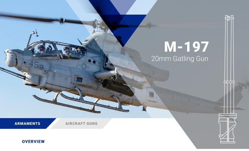
The 20mm M-197 produced by General Dynamics Ordnance and Tactical Systems is a lightweight, three-barrel version of the M61A1 Gatling gun intended for applications that require a lightweight, highly reliable weapon capable of firing up to 1,500 shots per minute.
